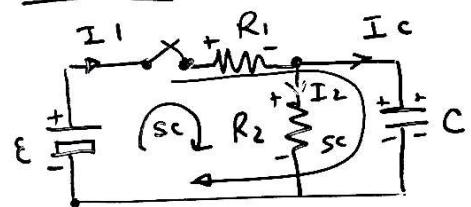
$$q(t) = \frac{ECR_2}{R_1 + R_2} + cte^* e^{-\frac{(R_1+R_2)}{R_1 R_2} \frac{t}{C}}$$
